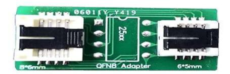
QFN8 adapter is a type of adapter used in electronics, which is used to test and program electronic components with QFN8 (Quad Flat No-Lead 8) substrate.
